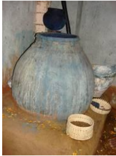
Left and below A large clay vat at the Institute of Rural Research, India, which stands in goats' dung to prevent fluctuations in temperature.
